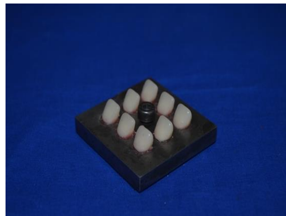
Figure 2. PMMA tooth attached to the mold
