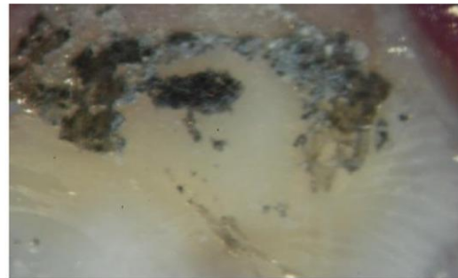
Figure 8. Mixed-mode failure observed in group A.
