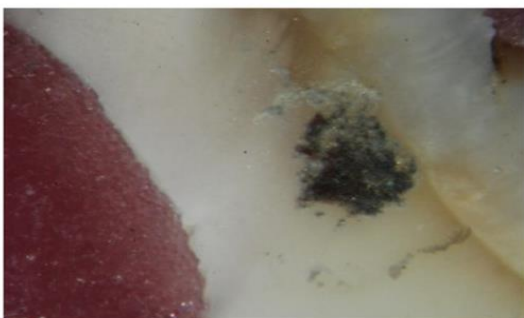
Figure 6. Cohesive-type failure in group A.
