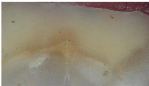
Figure 5. Adhesive-type failure observed in group B.
