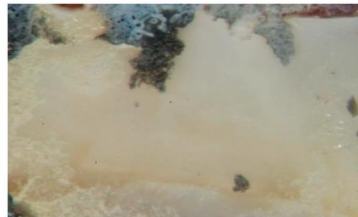
Figure 9. Mixed-mode failure observed in group B.
