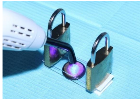
Figure 1. Construction of disc specimens
