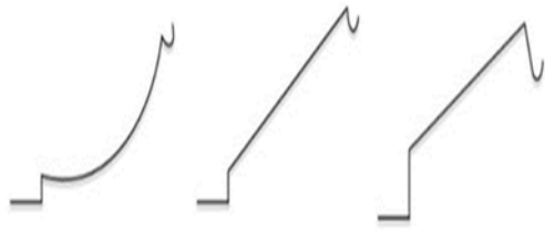
Figure 1. Different cantilever designs (activated). From the left: deep curve, tip back, and utility arch.
