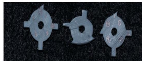
Figure 3. Examples of distorted calibration coupons observed during SLA 3D printing. The leftmost coupon exhibits incomplete formation of the top vertical strut, the middle coupon shows overall shape deformation with missing right-side and bottom struts, and the rightmost coupon has incomplete vertical struts on the top and left sides.
