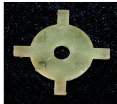
Figure 7. Completed calibration coupon printed using Dental SG resin for surgical guides (Formlabs, Somerville, MA, USA).
