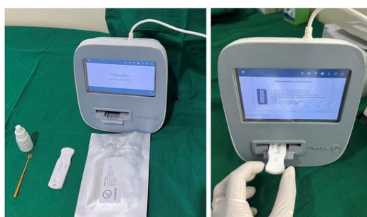
Figure 1. Tools and devices used in the study, including the saliva collection apparatus, buffer reagent, SpotSense CRP rapid testing device, and VIEWDx analyzer for quantitative evaluation
